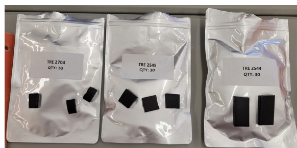
Figure 1. Experimental benzaldehyde lures formulated by Trécé, Inc., in a black polyvinyl chloride (PVC) proprietary matrix.
