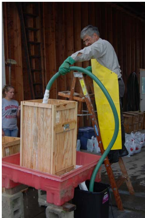
Left: Filling minibins with alternating layers of Cortland "data fruit" and Golden Delicious filler fruit. Although bins were 36 inches deep, six inches of headspace was left at the top to minimize splashing of treatment solutions. The full-size field bin in the rear was elevated on cement blocks for easier access to fruit. Right: A high-volume recycling drench is applied to fruit in a filled minibin while an assistant tracks time for the 30-second drench treatment.
