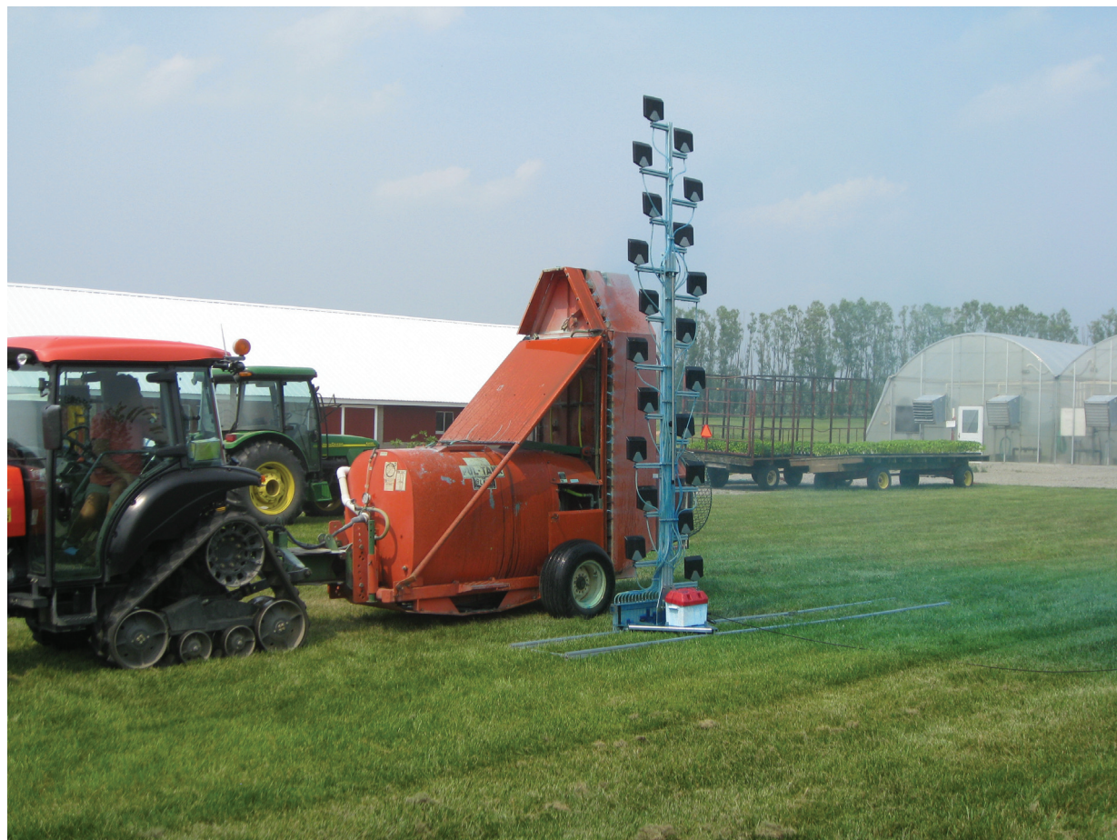
The patternator collects material from various locations from near the soil surface to what would represent the top of the tree.
