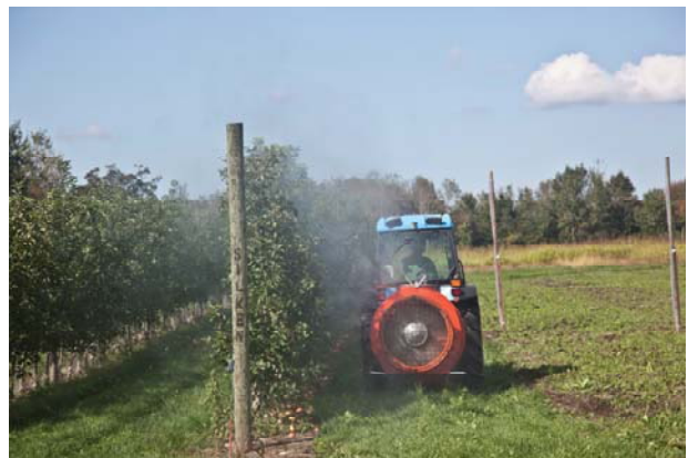
Figure 4. Airblast orchard sprayer in operation. Spray material clearly passes through the canopy. Likely, most will fall on the trees in the next row, but if weather conditions are undesirable, this material may move into non-target areas.
