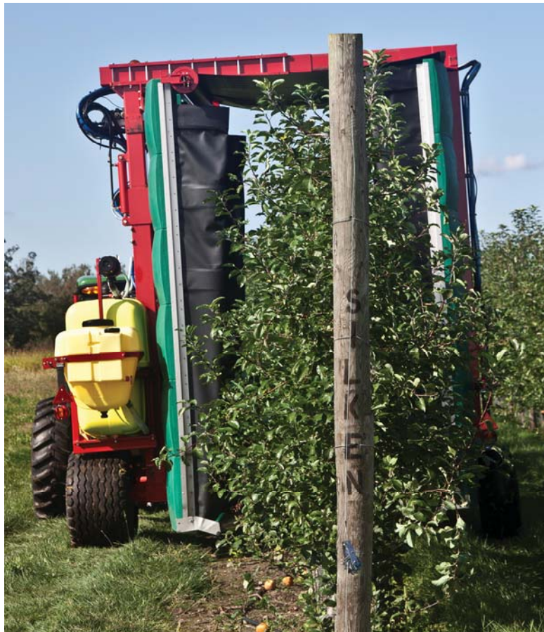
Figure 5. The Tunnel Sprayer directs material into the canopy from the outside and captures that which passes through the canopy.
