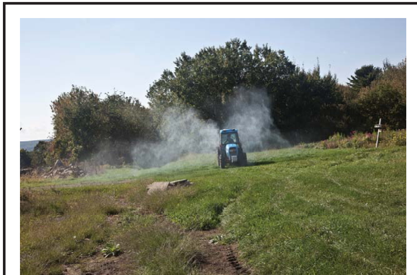
Figure 3. Even under nearly calm conditions, the airblast sprayer has the potential to create spray drift if it is not well calibrated.
